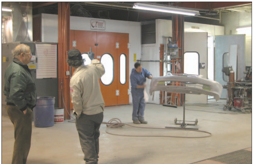
The shop has two downdraft spray booths and two prep stations.
